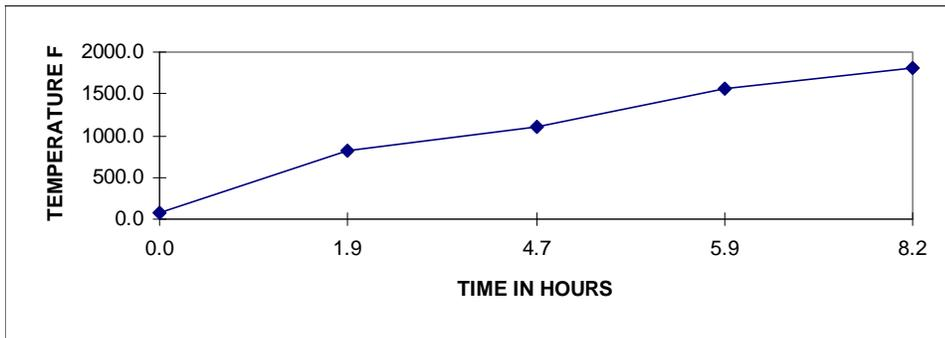
400°F per hour temperature rise until the kiln reaches 1000°F, then 100°F per hour until the kiln reaches 1100°F, then 400°F per hour until the final 250°F of the firing, then 108°F per hour until the setpoint is reached.
