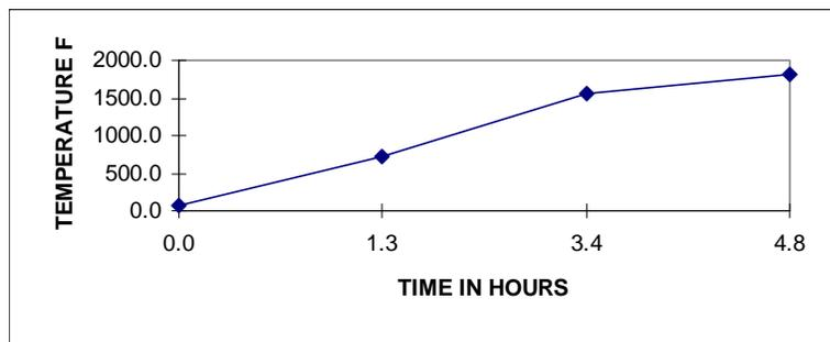
500°F per hour temperature rise until the kiln reaches 1100°F, then 400°F per hour until the kiln reaches the final 250°F of the firing, then 175°F per hour until the setpoint is reached. (Do not use this firing speed for firing above cone 05). The segment profile chart for MED-FAST is:
