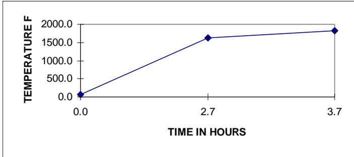
570°F per hour temperature rise until the kiln reaches 200°F below end setpoint (selected cone temperature), then 200°F per hour rise until the setpoint is reached. (Do not use this firing speed for firing above cone 05)
