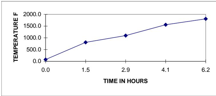
500°F per hour temperature rise until the kiln reaches 1000°F, then 200°F per hour until the kiln reaches 1100°F, then 400°F per hour until the final 250°F of the firing, then 120°F per hour until the setpoint is reached.
