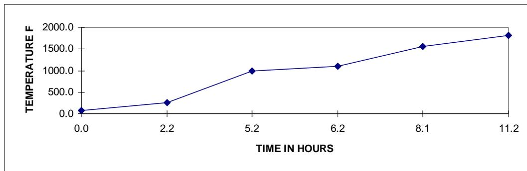
80°F per hour temperature rise until the kiln reaches 250°F, then 250°F per hour until the kiln reaches 1000°F, then 100°F per hour until the kiln reaches 1100°F, then 250°F per hour until the final 250°F of the firing, then 80°F per hour until the setpoint is reached.
