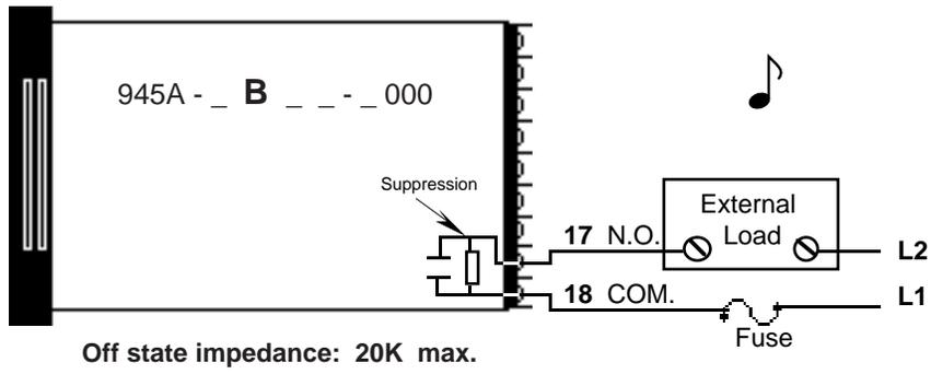
Figure 11 - Solid State Relay With Contact Suppression
