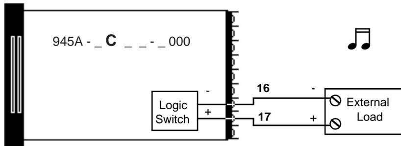
Figure 12 - Switched DC (Open Collector)
