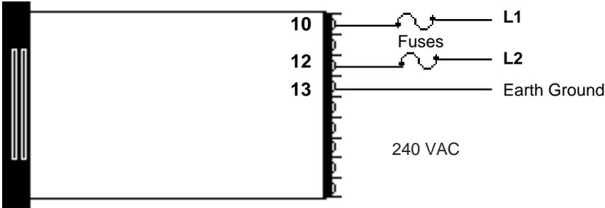
Figure 6 - 240 VAC Power Wiring
