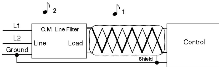
Figure 38 - Common Mode Filter Wiring
