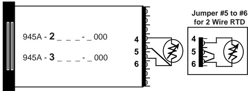
These input connections are also used in conjunction with T/C and RTD sensor types when using the remote set point input.
