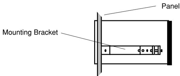
4. Insert the control chassis into its case and press the bezel to seat it. Turn the front panel screw 90° clockwise (CW) to lock the control in place.
