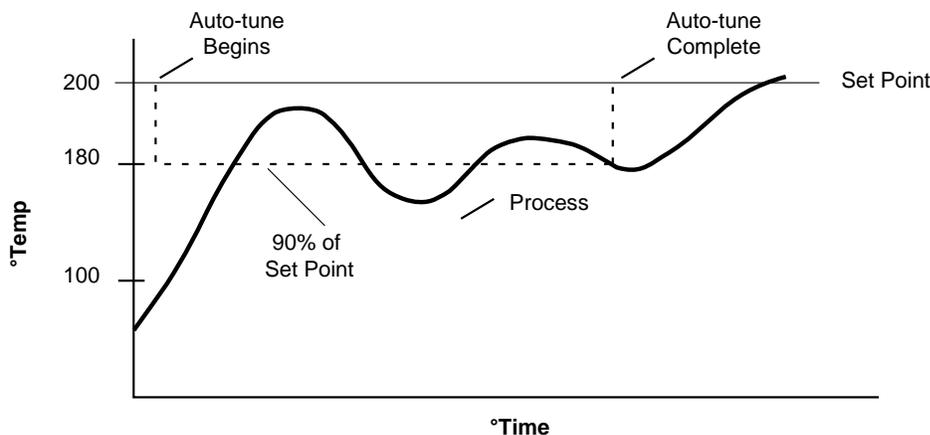
**Figure 33 - Auto-tuning at a Set Point of 200°F.**
