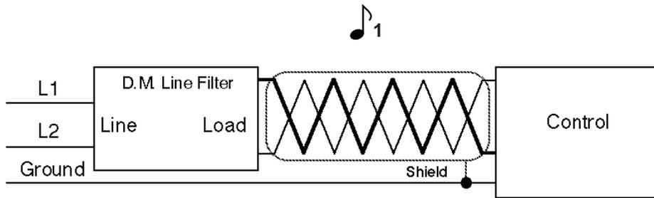
Figure 37 - Differential Mode Filter Wiring
