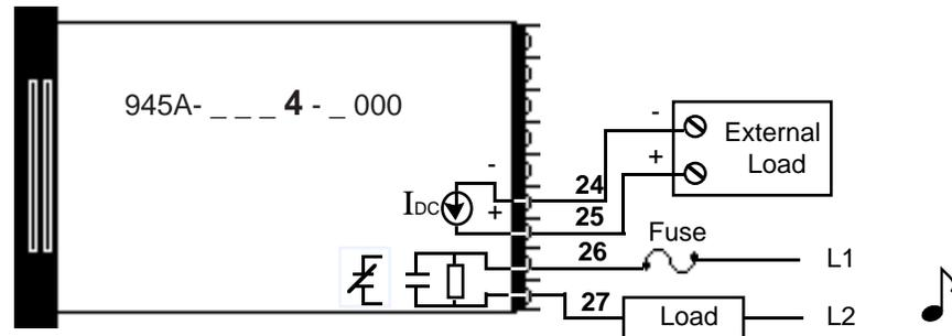
Load impedance: 10K min. for 4-20mA. Relay offstate impedance: 20K .
