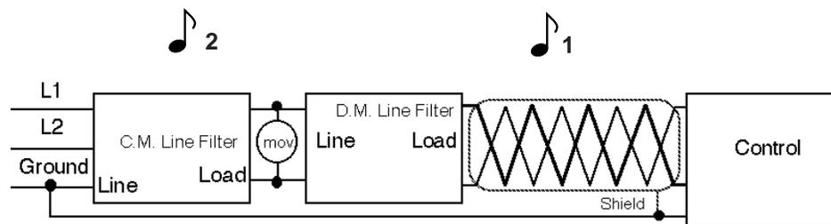
Figure 39 - Combination Differential/Common Mode Filter Wiring
