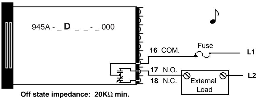
Figure 13 - 6 Amp Mechanical Relay
