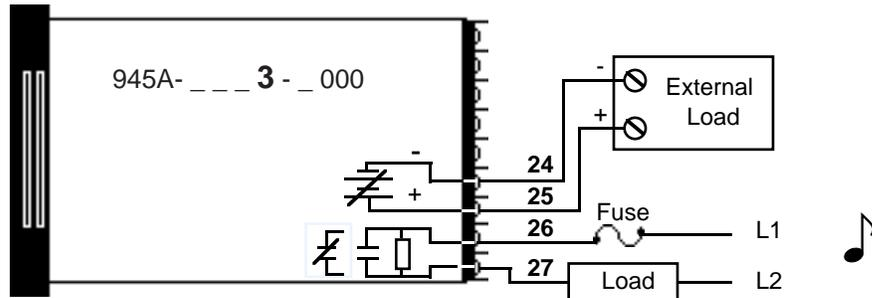
Load impedance: 10KΩ min. for 0-5VDC. Relay offstate impedance: 20KΩ.
