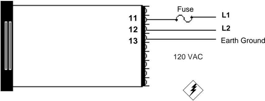
Figure 5 - 120 VAC Power Wiring
