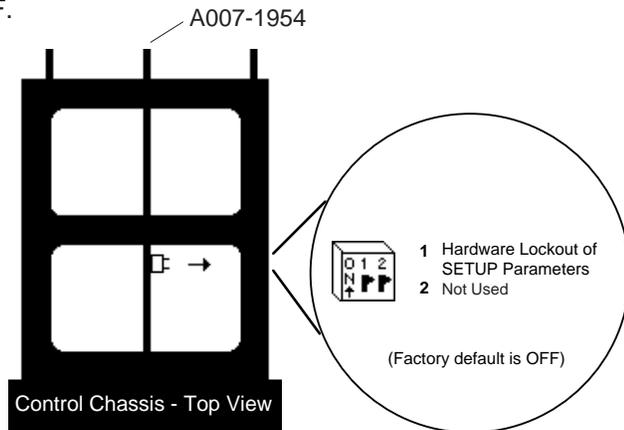
Figure 29 - DIP Switch Location and Orientation
