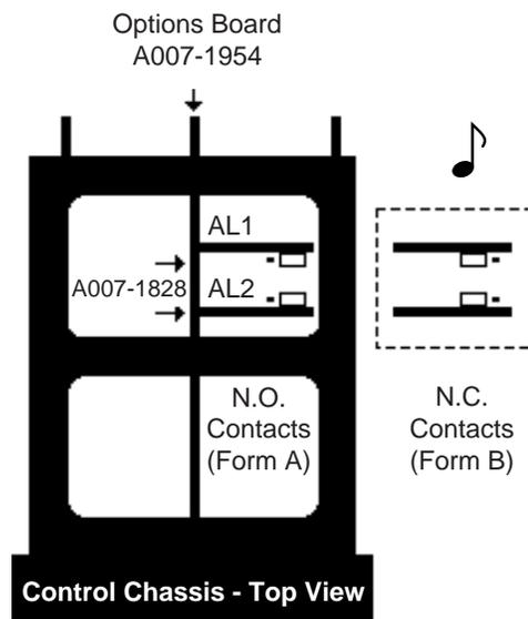
The alarm output de-energizes upon an alarm or power interruption to the 945's power supply. When you select **N.O. Contacts**, the contact is open when an alarm occurs. When selecting **N.C. Contacts**, the contact closes when an alarm occurs.
